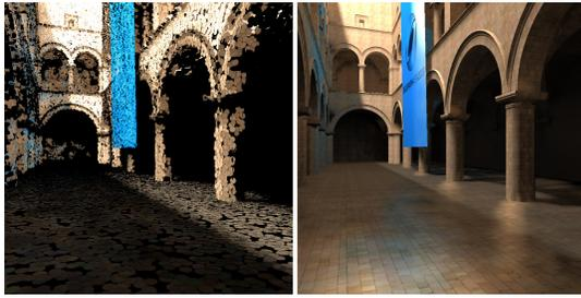
**Figure 8:** Final gathering for photon mapping. We first perform density estimation on the photon map (computed offline) for every point in our hierarchy (left). On the GPU, we then perform final gathering (right, note the glossy floor), which allows for interactive walkthroughs of photon mapped scenes (at 2 Hz) using bilateral upsampling with anti-aliasing from  $128 \times 128$  to  $1024 \times 1024$ .
