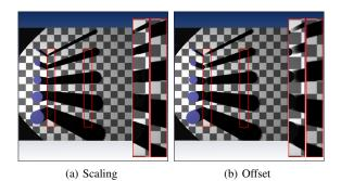
**Figure 4:** Difference of scaling f or subtracting an offset from d. (a) illustrates that scaling f sharpens the transition but also reduces filtering (shadows are sharper). (b) shows that subtracting an offset preserves convolution results but may exhibit reconstruction limitations near contact points (depending on M). Here we used a  $5 \times 5$  Gauss filter and
