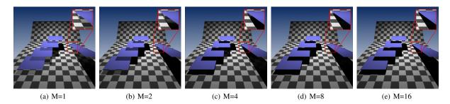
**Figure 6:** *Quality comparison for shadow test reconstruction using different number of Fourier series order M. All signals have been quantized to 8-bits per channel. When using a tightly fitted light frustum a single 8-bit RGBA texture usually faithfully reconstructs the shadow test. Note that ringing causes varying lightness in shadowed areas for small M.*
