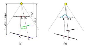
**Figure 2:** Fig. (a) illustrates shadow mapping. Point  $\mathbf{x}_1$  is lit, while point  $\mathbf{x}_2$  is in shadow. Fig. (b) depicts convolution using a filter kernel w. Filtering for a point  $\mathbf{x}$  is performed in shadow map space around point  $\mathbf{p}$ . See text for more information on  $\mathbf{q}$  and  $\mathbf{y}$ .
