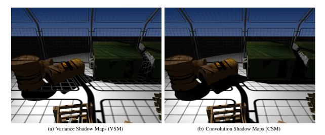
**Figure 9:** Comparison of VSMs (a) and CSMs (b). Scenes with high depth complexity such as this fence in front of other objects cause high variance in the convolution kernel. In such cases VSMs suffer from light leaking artifacts. (b) shows that CSMs correctly reconstruct the shadow function and render shadows without artifacts.
