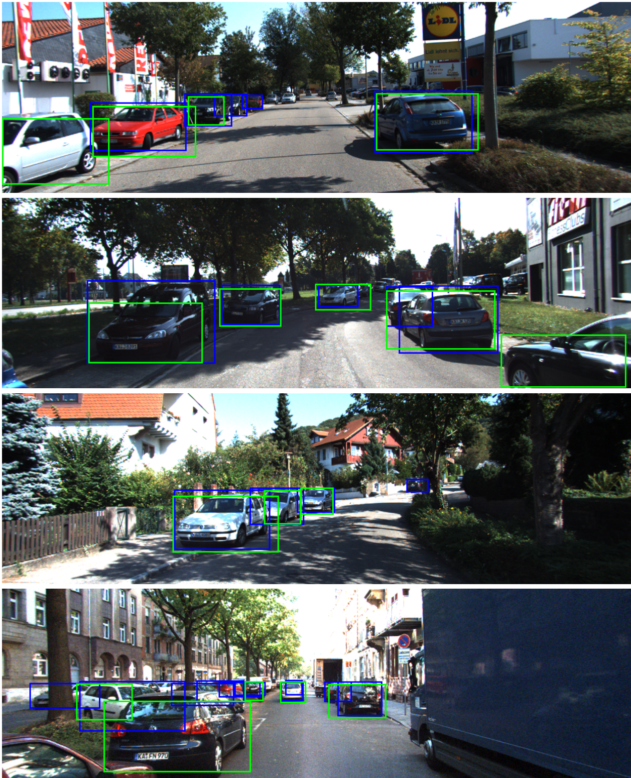
Figure 5: Visualization of object detections by SSOD on the KITTI [2] dataset. Green boxes show SSOD’s predictions and blue boxes show ground truth annotations. It can be seen that most of the cars with none to moderate occlusions are reliably detected. Cars with extremely heavy occlusions where only a small part of the car can be seen are sometimes missed.
