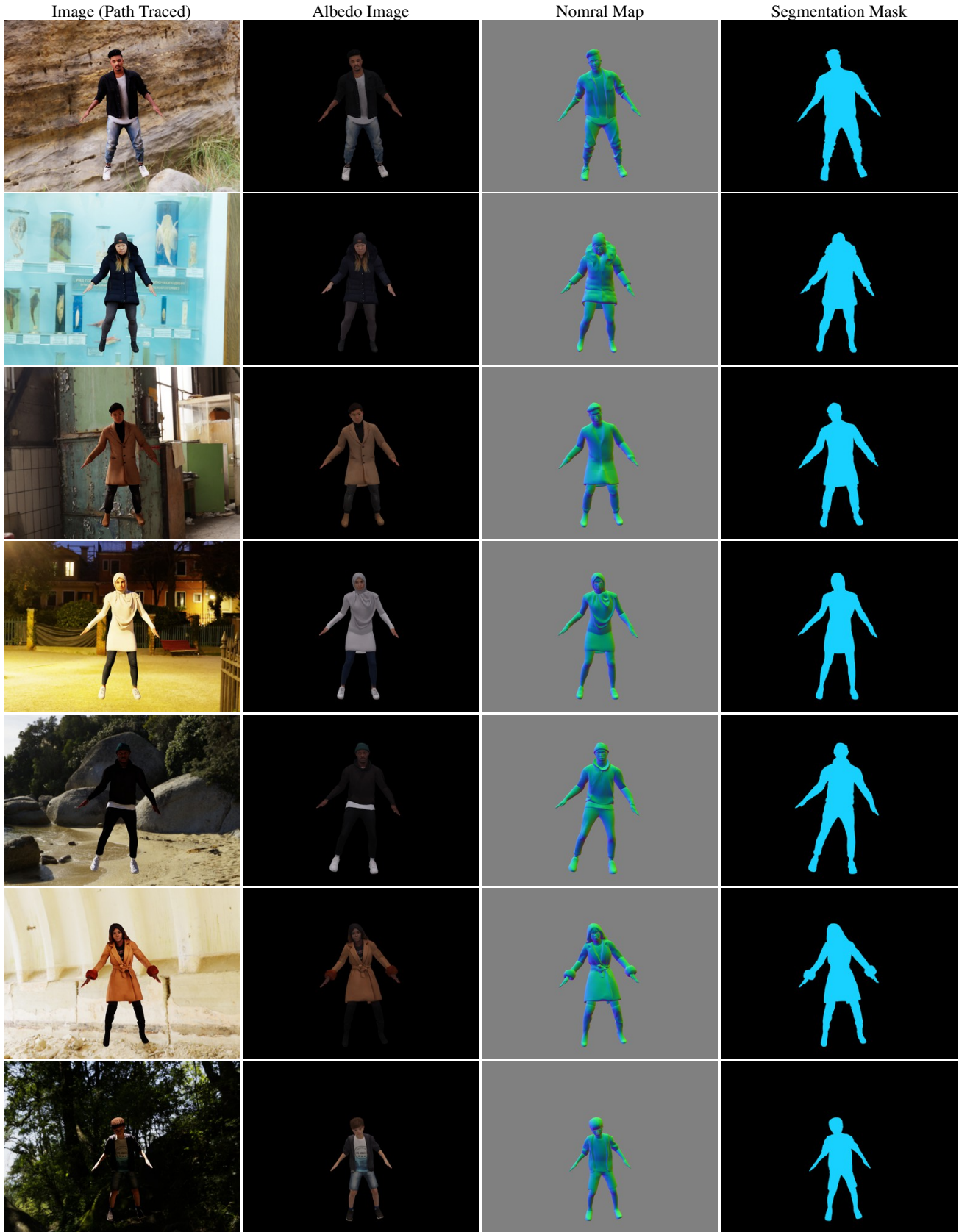
Figure 6. Example subjects from our proposed Relighting Humans dataset. We provide the ground-truth albedo map, normal map and segmentation masks as the ground truths.
