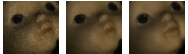
(a) Without noise reduction (b) Post-process bilateral blur (c) Our noise reduction method
