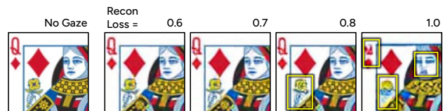
Figure 11. Reconstruction quality under varying loss thresholds. Outlined in recon_loss= 0.8, 1.0 are noticeable visual defects.
